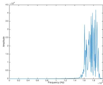
Figure 3: frequency spectrum plot ranges from 16 kHz to 19 kHz
